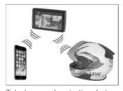
Telephone and navigation device cannot be connected with a helmet with a communication system at the same time. The telephone must be incorporated in the Bluetooth combination via the navigation device to enable both devices to be used at the same time. To do so, the navigation device is connected with the communication system as described (IIII) 100 per 1
